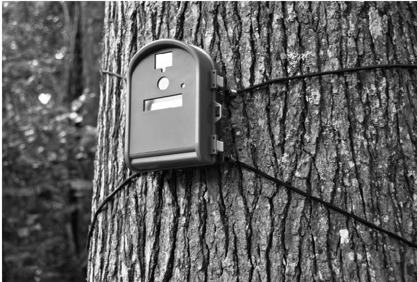
Figure 1: The included strap and stretch cords can be attached to the mounting points on the back of the camera and used to secure the camera directly to a tree.
