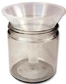
Figure 1: Example of a pitfall trap to be buried in the soil. Insects fall in the trap while walking. Trap can be filled with conservative liquid. Size: 10*15. Price: 10$.
